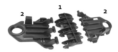
1) Hook side plate into the base bridge as picture shows. Pull it sideway forcibly till it moves into the final position.
