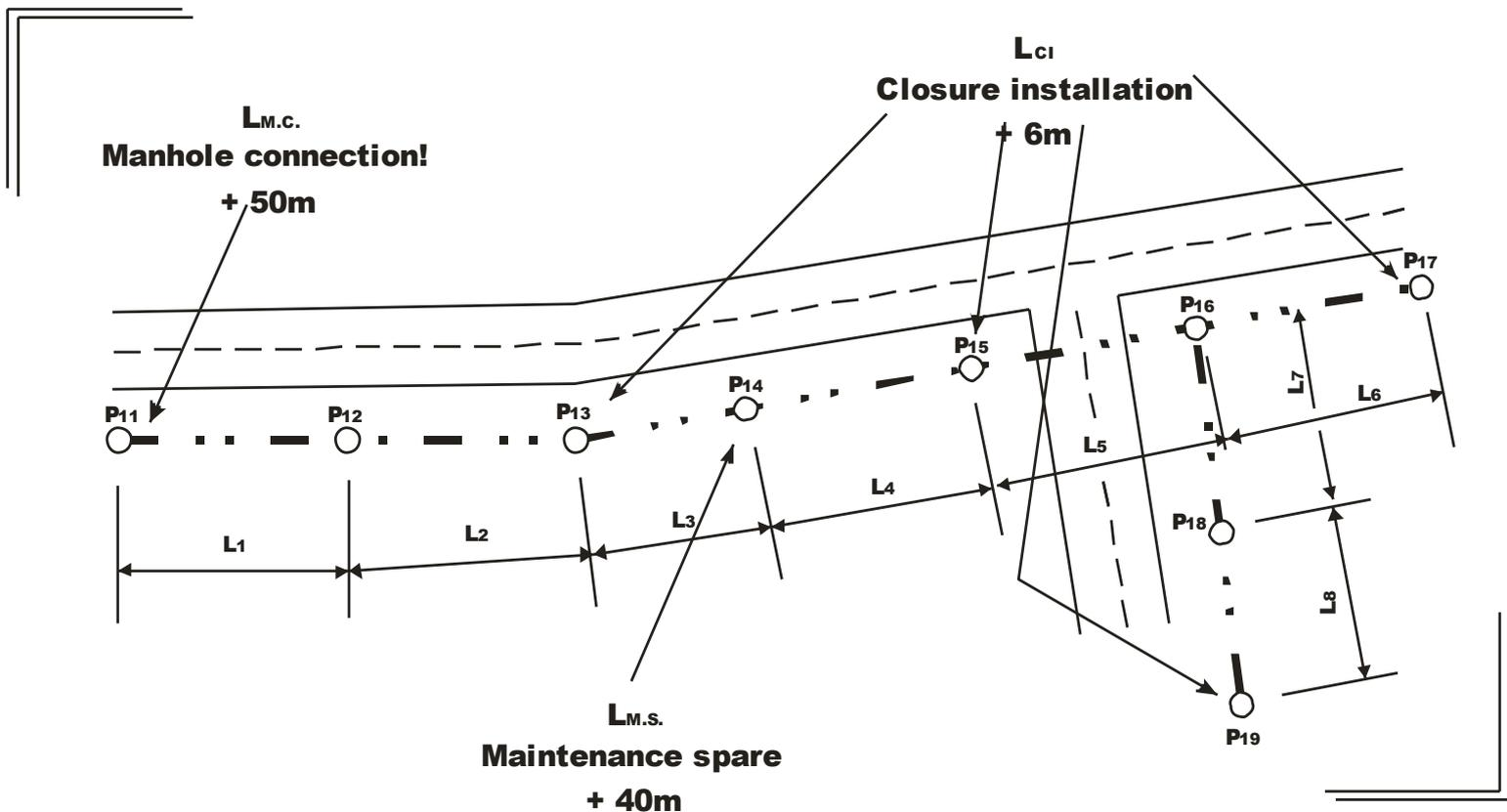
$L_{M.c.}$  = excess cable length for manhole connection
