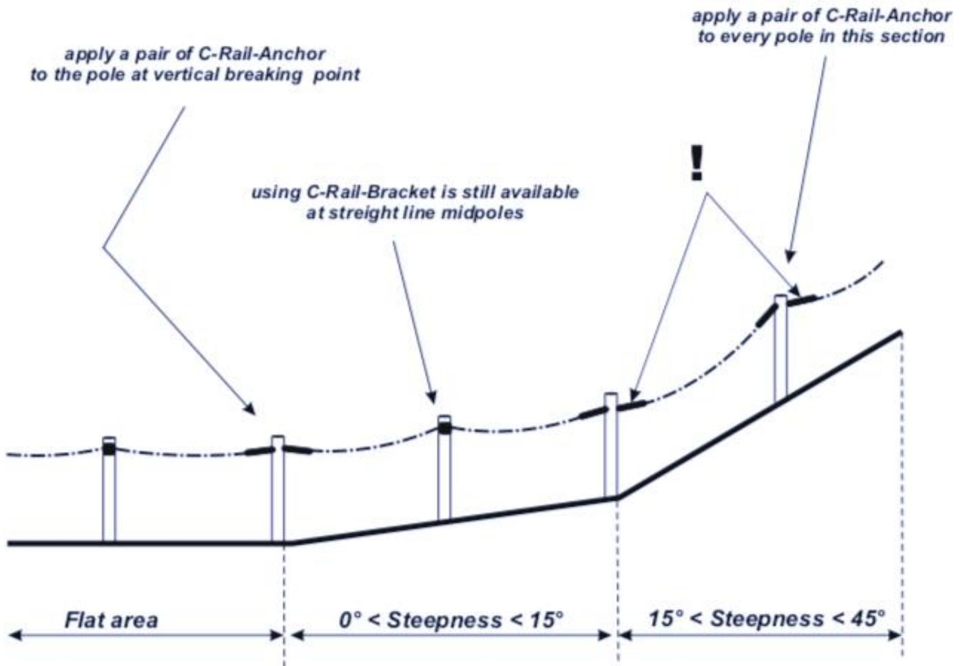
**!** - if steepness of hills exceeds  $15^\circ$ , the upper side C-RAIL-Anchors must be installed in combination with C-Rail-Hook-Base Mounting Plate. This addition supports angle mounting of C-Rail-Anchor
