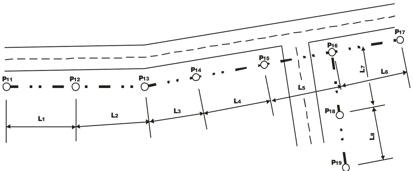
Length calculation:  $L_{mess} = (L1 + L2 + \dots + L8) \times 1,05$
